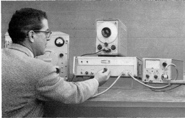
Fig. 1. New twt amplifier (center) increases signal generator levels to 1 watt in 1-12 gc range. With sweep-frequency generators internal modulation system can be used to provide constant power with frequency at levels up to 1 watt.
